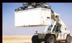
Example: Custom-built accommodation containers. Building optimised for -51° C.
