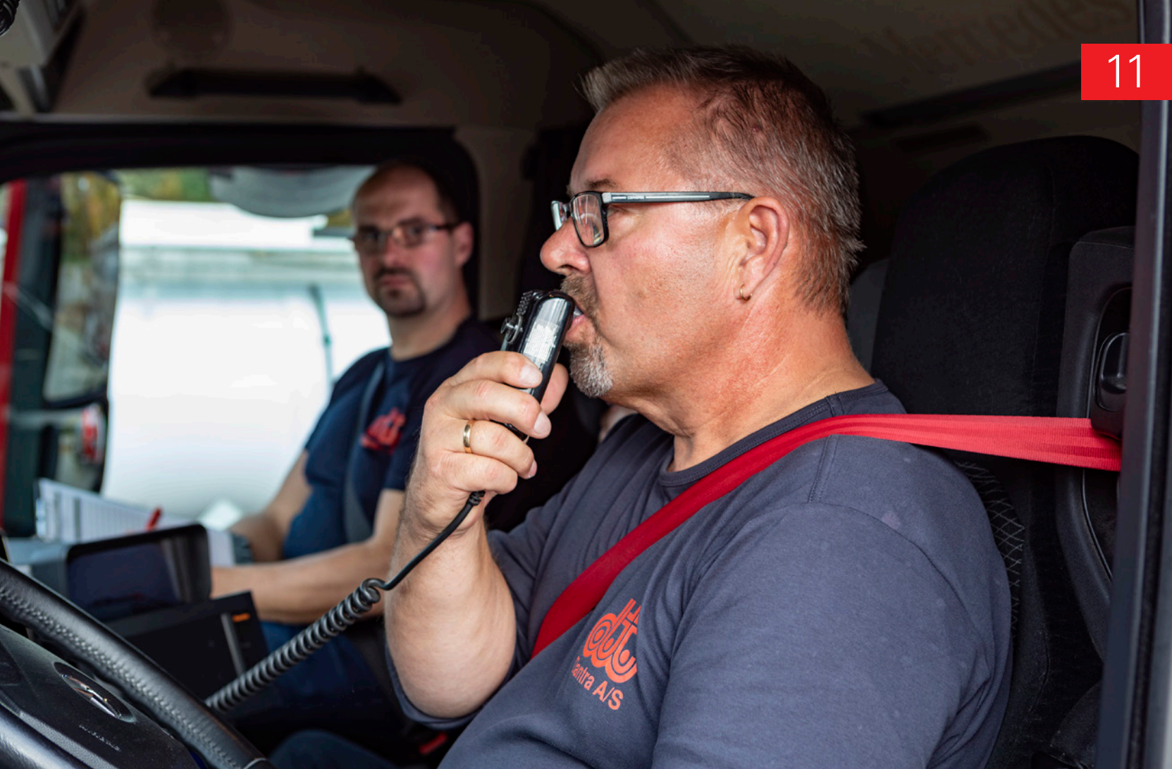
Driver and master driver operating an alcohol interlock device.
