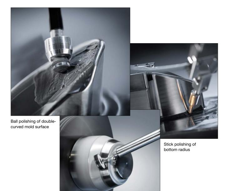
Polishing of a metal forming punch
